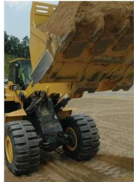
Under load, raise bucket to gauge how well it holds its position without drifting.
