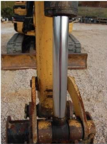
Cylinders should be free of nicks or dings. Oil on the chrome may indicate a reseal is needed.
