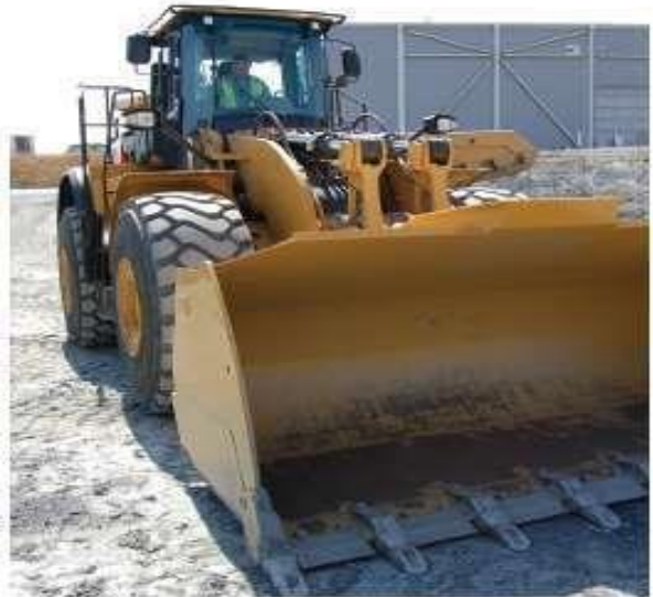
Look for wear on buckets and teeth. Reversible cutting edges are a plus.
