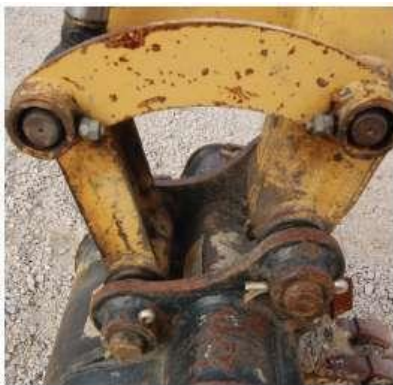
Bearings and bushings should have grease on them. While operating, look for any signs of flex or play.
